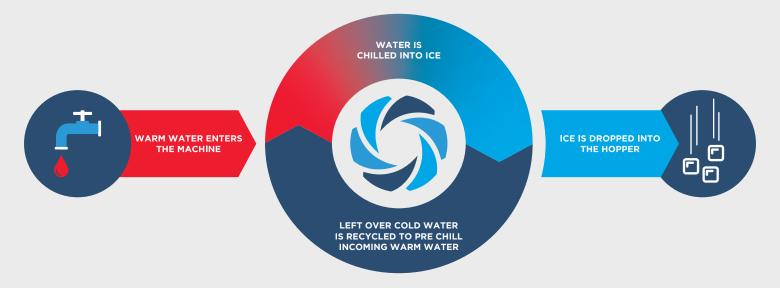
Cold Fusion, Everest's proprietary and patented technology, supercharges your ice maker. Instead of excess chilled water being dumped down the drain like our competitors, our technology recycles that water to be used to chill incoming warm water which creates more ice, using less electricity and extending the life of the ice maker.
